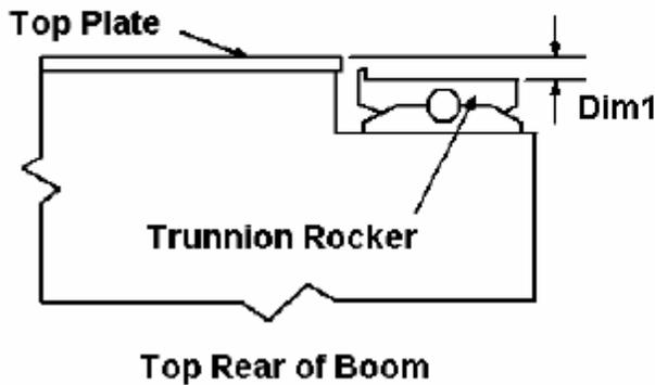
1. Place straight edge on top plate of boom section.
