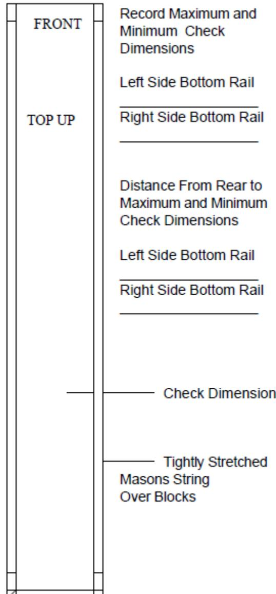
Record thickness of round or square gauge blocks \_\_\_\_\_
