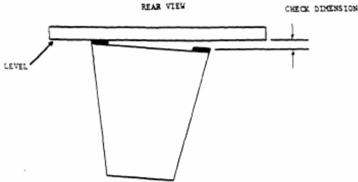
Record Check Dimensions as Twist \_\_\_\_\_
